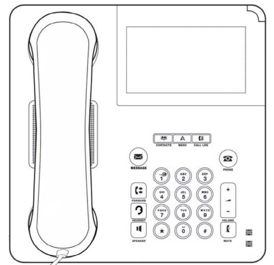
The phone supports 24 programmable call appearance/feature buttons. The labels for these are displayed in the scrollable main display along with icons for the status of the buttons.
