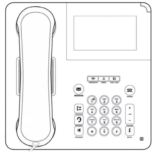
The phone supports 24 programmable call appearance/feature buttons. The labels for 6 of these are displayed in the main display and can be controlled by the adjacent buttons to the right. You can use the  $\blacktriangle$  up and down  $\forall$  arrow keys to scroll the display. You can also use the  $\blacktriangleleft$  left and right  $\blacktriangleright$  arrow keys to move through the button feature in pages of 6.
