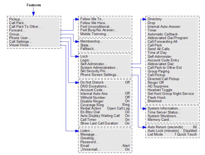
To exit the whole user menu and return to the appearance menu, press the **PHONE/EXIT** button or, if displayed, press the Exit soft key.
