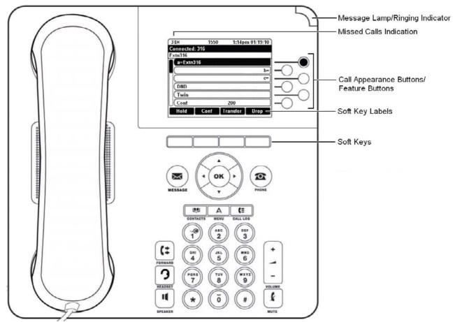
The phone supports 24 programmable call appearance/feature buttons. The labels for 6 of these are displayed in the main display and can be controlled by the adjacent buttons to the right. You can use the  $\blacktriangle$  up and down  $\nabla$  arrow keys to scroll the display. You can also use the  $\blacktriangleleft$  left and right  $\blacktriangleright$  arrow keys to move through the button feature in pages of 6.
