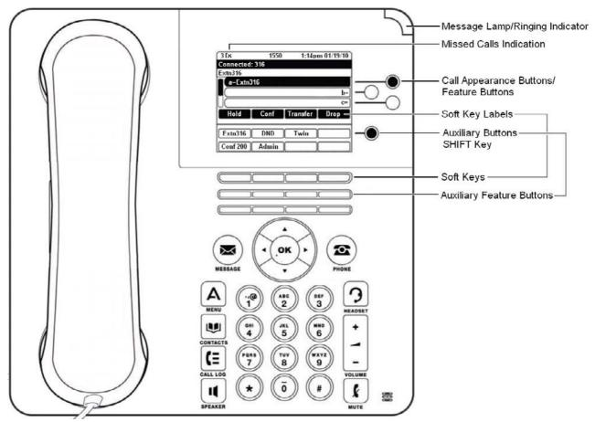
The phone supports 24 programmable call appearance/feature buttons. The labels for 3 of these are displayed in the main display and can be controlled by the adjacent buttons to the right. You can use the  $\blacktriangle$  up and down  $\P$  arrow keys to scroll the display. You can also use the  $\P$  left and right  $\blacktriangleright$  arrow keys to move through the button feature in pages of 3.
