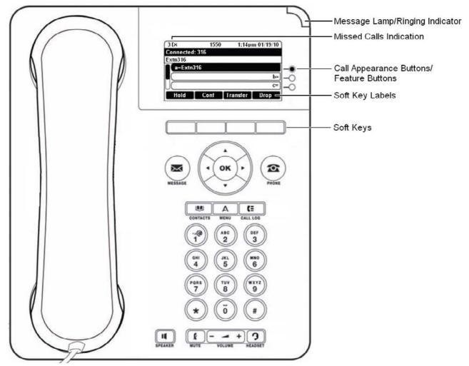
The phone supports 12 programmable call appearance/feature buttons. The labels for 3 of these are displayed in the main display and can be controlled by the adjacent buttons to the right. You can use the  $\blacktriangle$  up and down  $\P$  arrow keys to scroll the display. You can also use the  $\P$  left and right  $\blacktriangleright$  arrow keys to move through the button feature in pages of 3.
