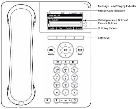
The phone supports 12 programmable call appearance/feature buttons. The labels for 3 of these are displayed in the main display and can be controlled by the adjacent buttons to the right. You can use the  $\triangle$  up/down  $\nabla$  keys to scroll the display. You can also use the  $\triangleleft$  left/right  $\triangleright$  keys to move through the button feature in pages of 3.
