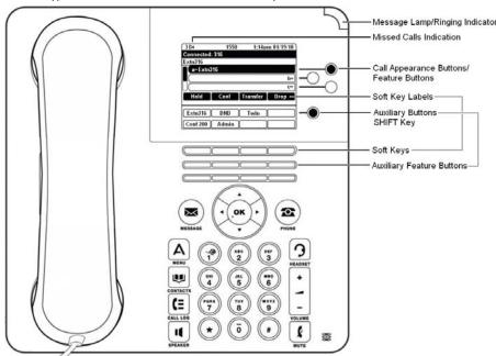
The phone supports 24 programmable call appearance/feature buttons. The labels for 3 of these are displayed in the main display and can be controlled by the adjacent buttons to the right. You can use the  $\triangle$  up/down  $\nabla$  keys to scroll the display. You can also use the  $\triangleleft$  left/right  $\triangleright$  keys to move through the button feature in pages of 3.
